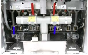
Ensure the filter pan is fully seated on the male connection (left, above) when it slides into place.
